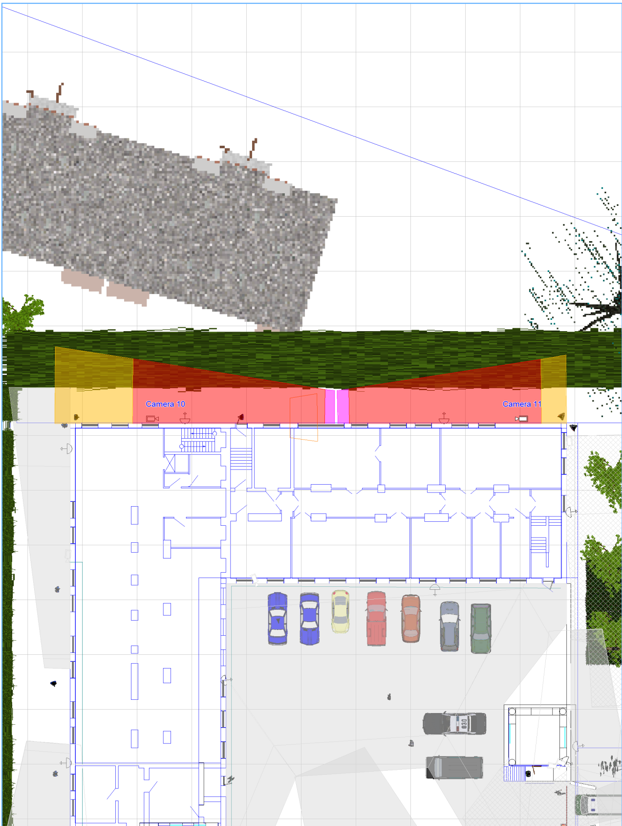
Fig.29. View area projections of cameras of the Group Perimeter top
